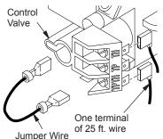
Figure 19 - Connecting Wire Terminals
